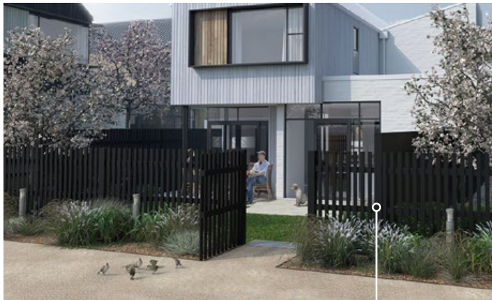
1.2m height and 50% open / permeable at front yard
